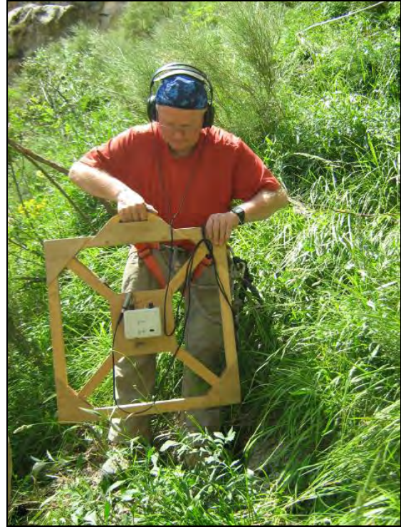
Identification of the magnetic field direction sent by the transmitter located underground [photo. Ph. Audra]
